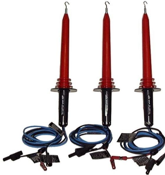
The 5KVP comes as a set of three probes. Each probe is 14 inches long and weighs less than a pound. The fully extended length of the leads and probes is 7 feet.
